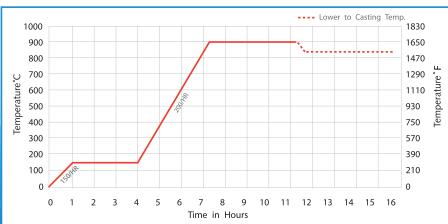
Do not remove flasks from furnace to cast until they have been held at casting temperature for a minimum of 1 hour. If held for less than 1 hour, the core of the flasks will be at a much higher temperature than the digital temperature display states, and may result in metal mould reaction.
